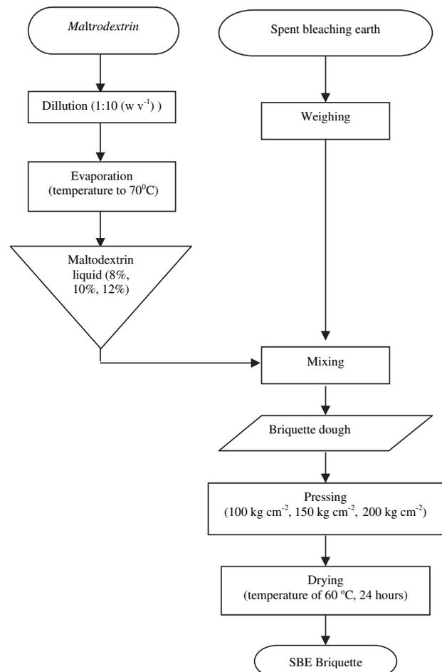
Fig. 2 – The procedure of SBE briquetting.
