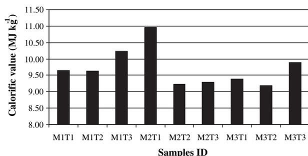
Fig. 5 – Calorific value of SBE briquettes.
