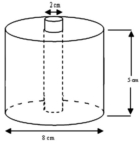
Fig. 1 – SBE briquette mold.
